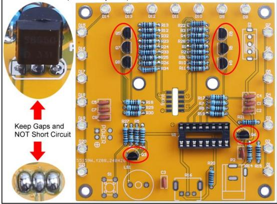
Step 8: Install 8pcs TO-92 S8550 Transistor at Q1-Q8. The arc on the PCB correspond to the arc of the components. Adjacent pins must not be short circuited.
