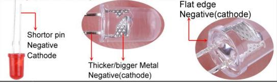
Step 23: Install 12pcs 3mm Yellow LED at D0,D5,D10,D15,D20,D25,D30,D35,D40, D45,D50,D55 on PCB another side. Note: the shorter pin connect to flat edge or round pad as shown.
