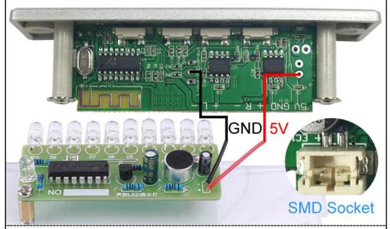
Method-3 for DIP and SMD Socket Version Bluetooth Module.
