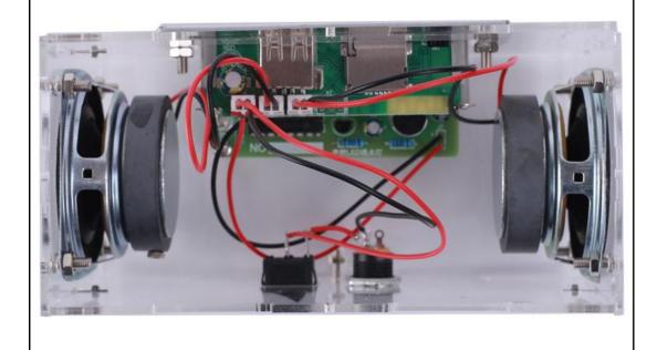
Step 28: Assemble 6pcs acrylic panels by 12pcs M2\*10mm Screw and 12pcs M2 Nut. Please be patient when installing the screws.
