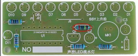
Step 4: Install 1pcs DIP-6 IC CD4017 at U1. There is a mark(notch) on one end of the IC and there is a mark(curved silk screen printing) on PCB where the IC can place on. These two marks are corresponding to each other and are used to specify the
