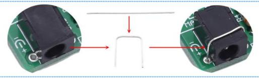
Step 10: Fix the power socket with the extra pins of the resistor.
