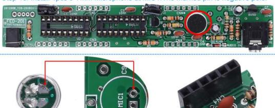
Step 16: Install 5pcs 2.54mm Female Socket 1\*6Pin at CN1-CN4,CN\*.
