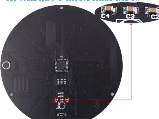
Step 7: Install 3pcs 0.1uF 0805 SMD Capacitor at C2~C4.
