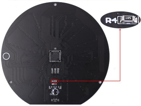
Step 5: Install 1pcs 1Mohm(105) 0805 SMD Resistor at R4.
