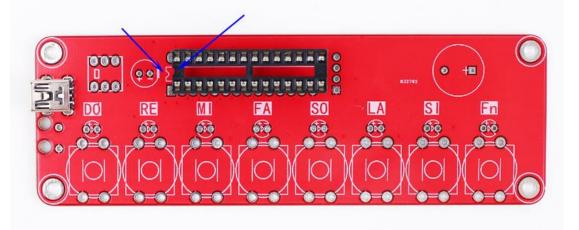
Step 3: Install 1pcs DIP-28 STC15W408AS at U1 on IC Socket.Must not be installed reverse, otherwise it will not work properly.Note:Users can also install this chip last.
