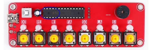
Step 10: Install 1pcs red button cap on Self-Locking Switch and 8pcs yellow button cap on button.
