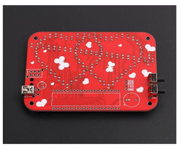
Step 2: Install Mini USB and 2pcs button on other side of PCB.
