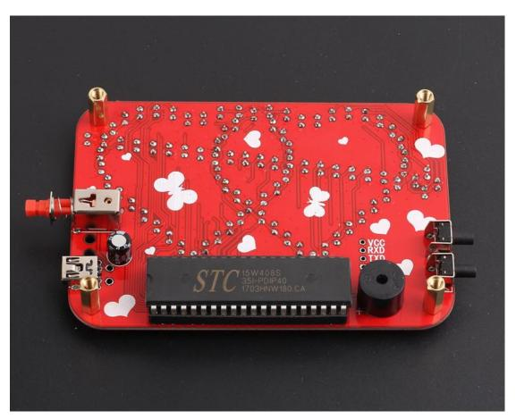
Step 6: Install Copper Pillar and test!
