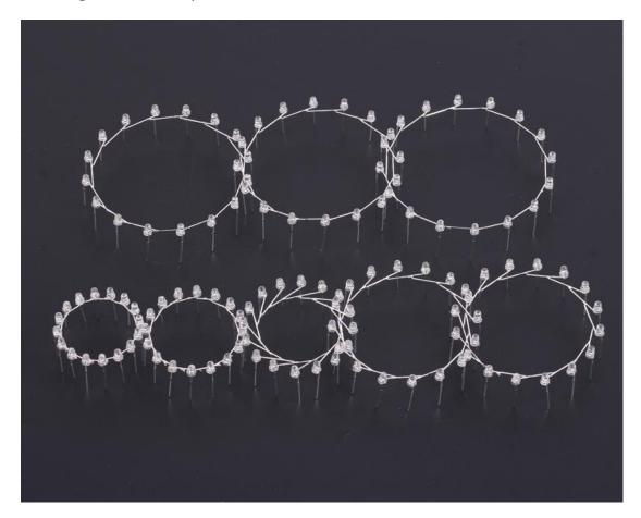
Step 12: Install the 6th Ring as the 1st Layer LED.Bend the pins slightly. First fix a pin, and then fixed the pin on opposite position. Use pliers to bend the tip of the pin if not convenient to install.
