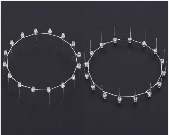
Step 11: Install the 2nd Ring to the 6th Ring total 8pcs LED rings as Step 10.
