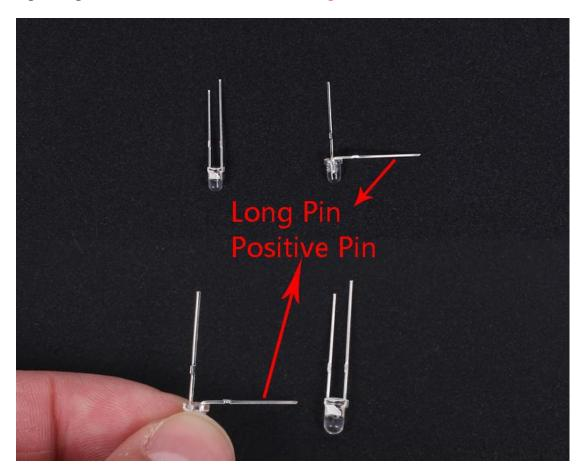
Step 10: Install the 1st Ring LED with Acrylic welding template. Short pin(Negative pole) outward, Longer pin(Positive pole) interconnection.
