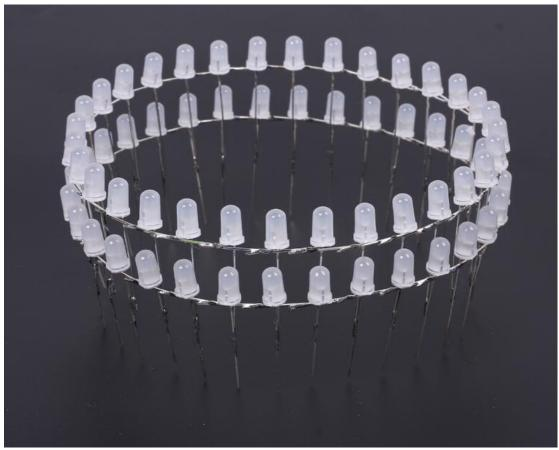
Step 13: In accordance with the above method, made into two 4-layer LED dot lattice.
