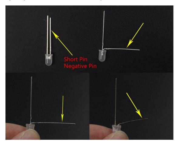
Step 8: Install the 1st layer LED with Acrylic welding template. Short pin(Negative pole) outward, Longer pin(Positive pole) interconnection.
