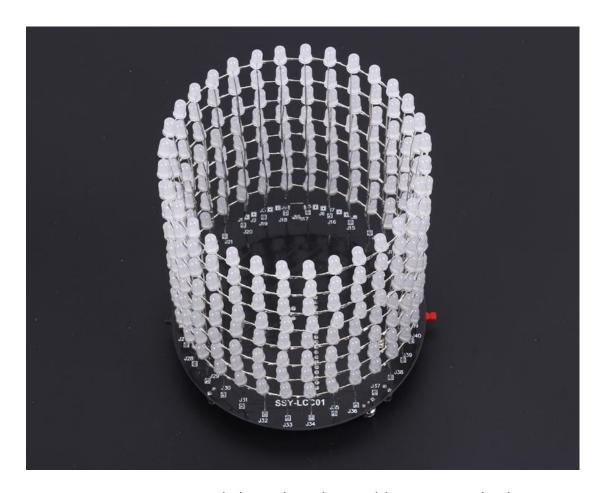
Step 16: Connect each layer by white cable on J1-J8. The bottom is the first layer.
