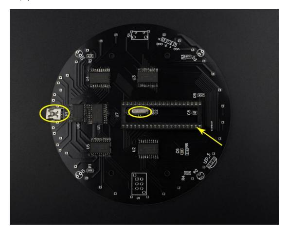
Step 5: Install 4pcs 5mm LED on D1-D4;1pcs Button on S1;1pcs Self-Locking Switch on S;1pcs Infrared Receiver on LED\_S;1pcs 4P Male Pin on X.
