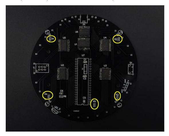
Step 4: Install 1pcs Crystal Oscillator on Y1;1pcs 40Pin IC Socket on U7;1pcs MINI USB Socket on P1.Install in the above order!
