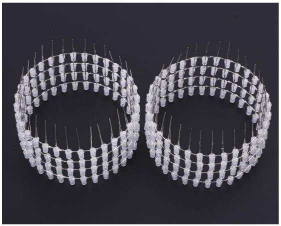
Step 14: Splicing 2pcs 4-layer LED ring. Mainly use the thumb. In strict accordance with the above method. Solder wire access from inside.
