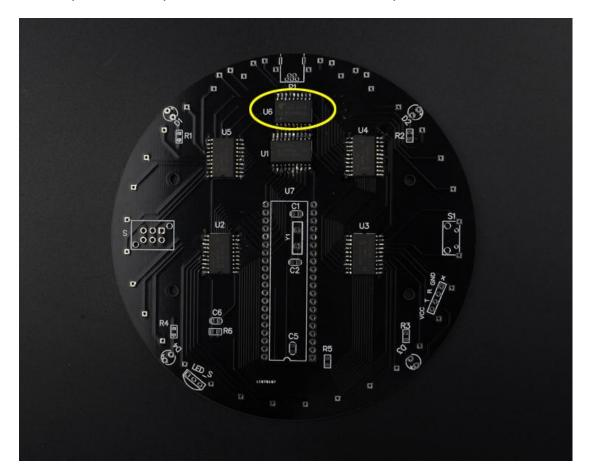
Step 2: Install 2pcs 27pf capacitor on C1,C2 and 1pcs 47pf on C5,1pcs 10uf on C6.
