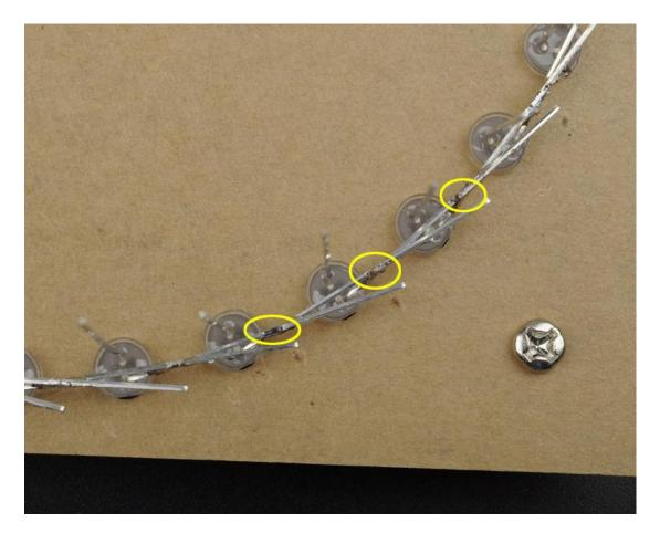
Step 9: Test. Check with a multimeter if each LED can be lit.Replace the damaged LED in time.And then cut off excess pins.
