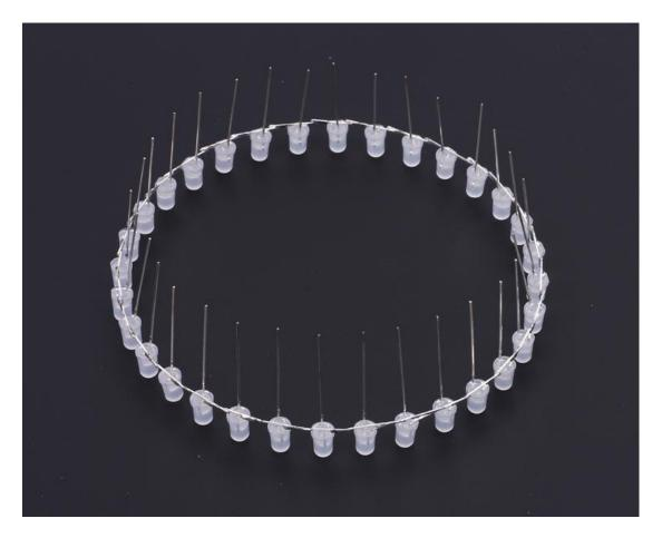
Step 12: Splicing two LED rings.Note the caution points marked below.Please wear gloves to operate or wrap your fingers with cloth,Mainly used index finger.Avoid being scalded
