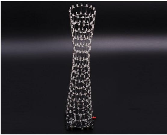
6).Step 35:Install spire.There are 16pcs LED on the 16th layer of Tower main body and 5pcs LED on the 1st layer of spire.So there are 3pcs LED on the 16th layer between 2pcs LED on the 1st layer of spire,and others just have 2pcs LED.Please see picture,you can understand clearly.
