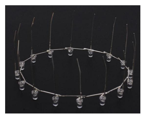
2).Step 31:Put some tin on the root of positive pole in order to fix next layer LED.
