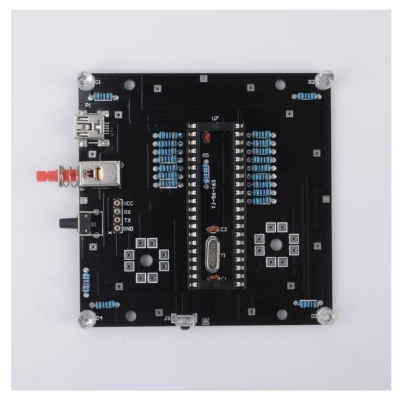
6).Step 6:Install 16pcs Round Female pin on other side of PCB on J1-J16 pad.It is use for LED
