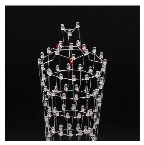
8).Step 37:Install the 4th layer of spire.Negative pole connect to the negative of the 3rd layer and positive pole connect to the positive of the 3rd layer of spire.
