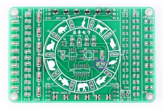
Step 15:Install 1pcs S9014 SMD J6 SOT-23 Transistor at Q1.
