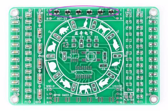
Step 8:Install 6pcs SMD 0603 Network Resistor at 8P4R 0603.Due to its very small pin pitch, please be patient and install.
