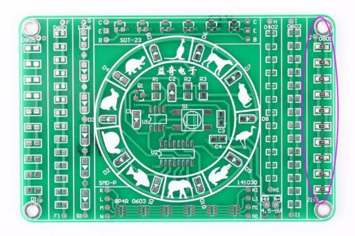
Step 2:Install 14pcs SMD 0603 Resistor at 0603 I.
