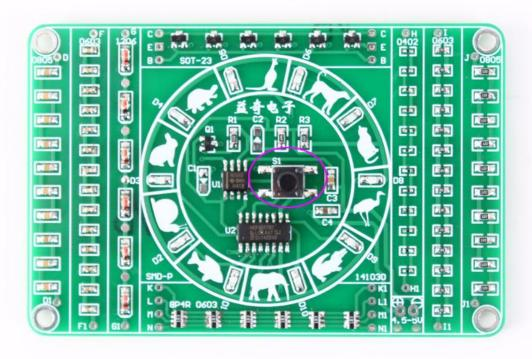
Step 19:Install 2pcs 22uF SMD 0805 Capacitor at C1,C2.
