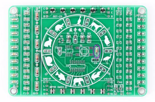
Step 14:Install 1pcs 0.1uF SMD 0805 Capacitor at C4.
