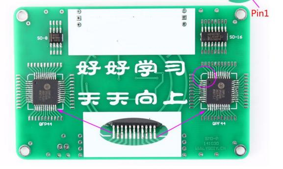
Step 11:Start installing the components in the practice area.Install 1pcs 470K SMD 0805 Resistor at R2.
