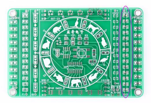
Step 3:Install 12pcs SMD 0402 Resistor at 0402 H. Note:0402 components are very small, please be patient to complete the installation.
