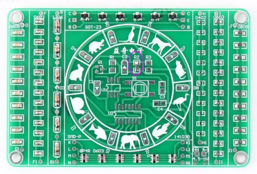
Step 12:Install 2pcs 1.2K SMD 0805 Resistor at R1,R3.
