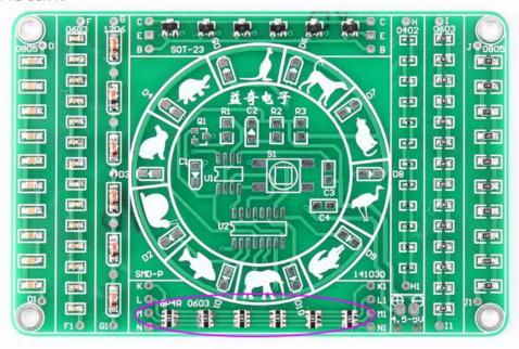
Step 9:Install 1pcs SOP-8 IC at SO-8 and 1pcs SOP-16 IC
