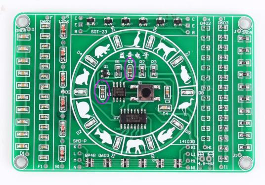
Step 20:Connect DC 4.5V-5.0V to do a test.
