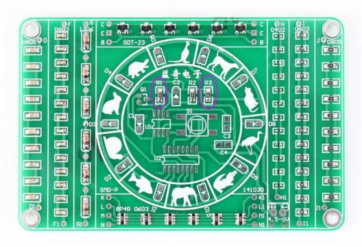
Step 13:Install 1pcs 0.01uF SMD 0805 Capacitor at C3.
