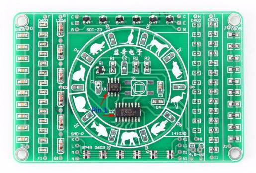
Step 17:Install 10pcs Red SMD 0805 LED at D1-D10. Note: LED distinguishes between positive and negative, can not be installed reverse, otherwise the LED will be damaged and will not work properly. Methods to identify positive and negative:One end of the green mark is the negative. Or test positive and negative by multimeter.
