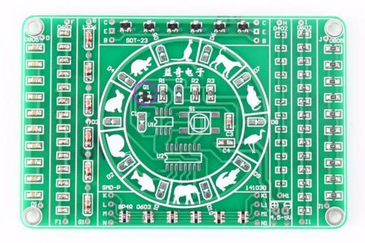
Step 16:Install 1pcs SOP-8 NE555 at U1 and 1pcs SOP-16 HEF4017 at U2.But pay attention to the installation direction.
