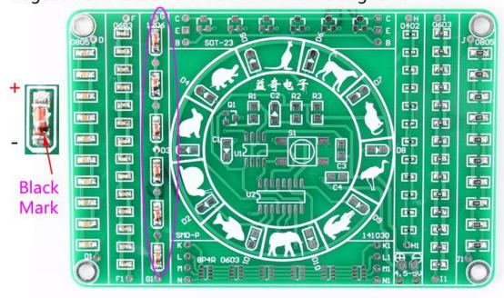
Step 7:Install 6pcs SMD J6 SOT-23 Transistor at SOT-23.
