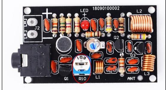
Step 11: Install 1pcs KF-301-2P Connector at J2.
