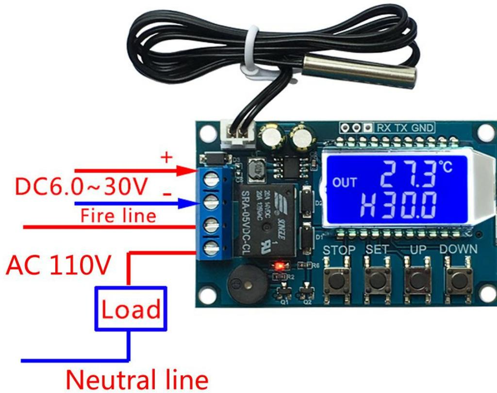
LCD will display 'h' in last line and last bit if turn ON delayed start.
