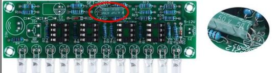
Step 17: Install 1pcs 100uF Electrolytic Capacitor at C2. The PCB silk screen printing features a white marking indicating where the negative (cathode) lead can be inserted. It's important to note that the shorter lead is the negative (cathode) pole, and the capacitor must be placed horizontally.
