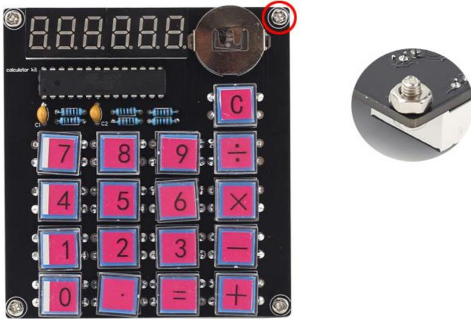
Step 14: Peel off the protective film on the surface of the acrylic case.
