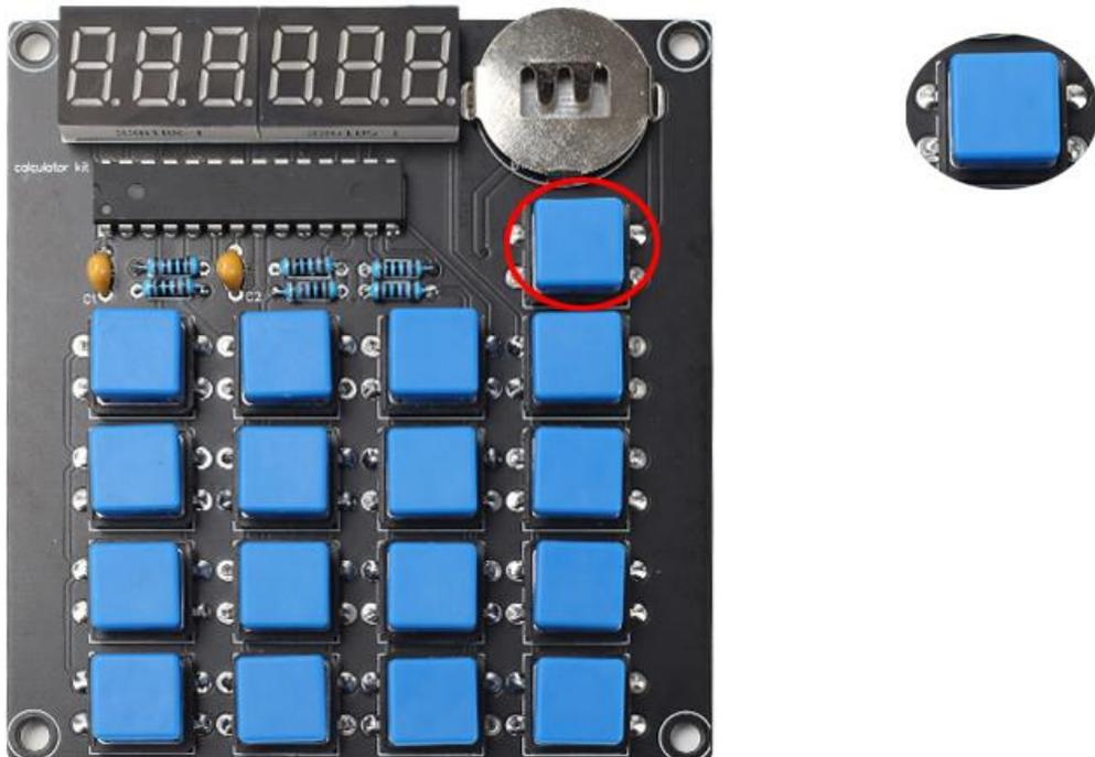
Step 11: Tear off the small label with tweezers and stick it on the corresponding blue keycap.
