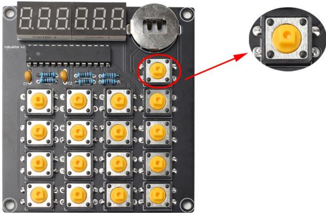
Step 10: Install blue keycaps on each of the 17 switches.
