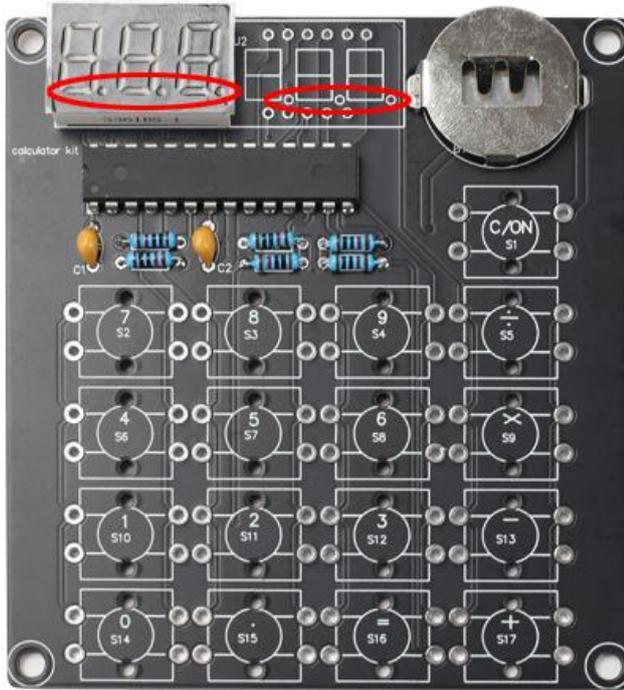
Step 8: Install a digital tube at U2, pay attention to the installation direction.
