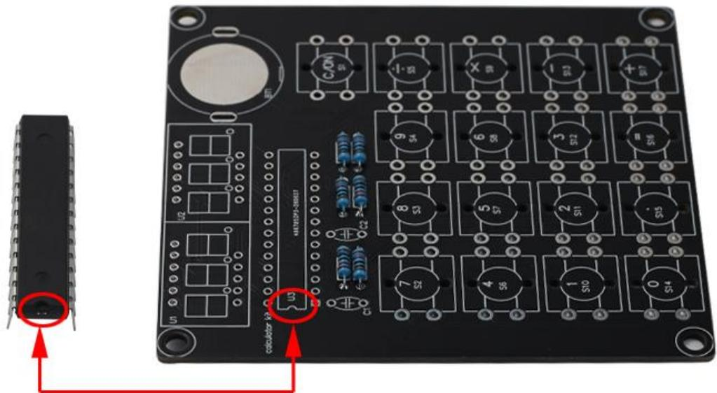
Step 3: After the MEGA328 is placed, select a lead to solder, and after soldering, solder the diagonally opposite pins. After adjusting the position, solder the remaining pins in sequence.
