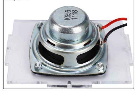
Step 40: Install Speaker Acrylic Board by 4pcs M3\*8mm Screw and 4pcs M3 Nuts. Pay attention to the placement of wires and do not place them between the speaker and PCB to avoid affecting the installation of acrylic board.
