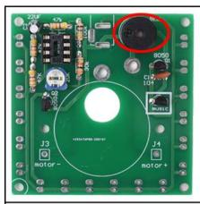
Step 23: Install 1pcs Passive Buzzer at BELL.
