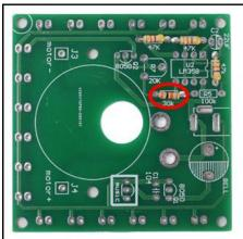
Step 15: Install 1pcs 30Kohm Metal Film Resistor at R6 on Main PCB.
