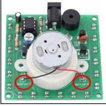
Step 28: Install 1pcs DC3V-9V JS-30 DC Motor at motor. It is a DC motor, so there is no need to distinguish between positive and negative.
