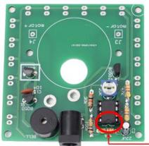
Step 25: Install 1pcs DIP-8 LM358 at U2. There is a mark on one end of the LM358 and there is a mark on IC Socket where the LM358 can place on. These two marks are corresponding to each other and are
