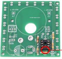
Step 17: Install 1pcs DIP-8 IC Socket at U2.
