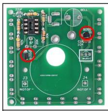
Step 19: Install 2pcs TO-92 S8050 Transistor at Q1,Q2.Pay attention to the installation direction.
