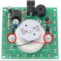
Step 29: Fixed motor by 2pcs M3+10mm Screw and 2pcs M3 Nut.
