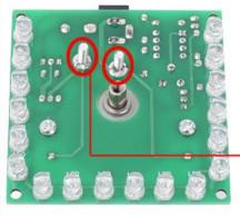
Step 30: Fix 2pcs M3+10mm Screw at 3mm holes by solder.(Note:Please do not use nuts to fix!)
