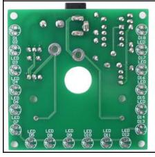
Step 26: Pay attention to mark of LED silk screen which can distinguish positive and negative poles. The longer pin is inserted into positive poles pad.
