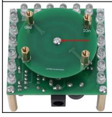
Step 36: Fixed Bottom Round PCB on motor shaft by 1pcs M3+6mm Screw.
