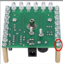
Step 31: Install 4pcs M3+25mm Copper Pillar and 4pcs M3+6mm Screw on Main PCB as a stand.
