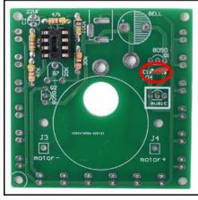
Step 18: Install 1pcs 0.1uF 104 Ceramic Capacitor at C1.
