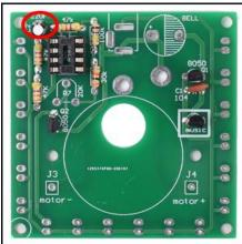
Step 21: Install 1pcs 22uF 25V Electrolytic Capacitor at C2.Pay attention to distinguish between positive and negative.
