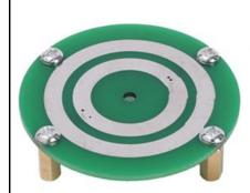
Step 35: Install 4pcs M3+10mm Copper Pillar and 4pcs M3+6mm Screw on Bottom Round PCB which has two ring. The ring and Copper Pillar are also used as circuits.
