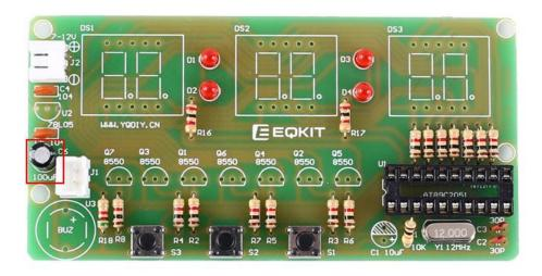
Step 14:Install 1pcs 10uF/25V Electrolytic Capacitor at C1.Pay attention to the installation direction and the shorter pin is negative pins.
