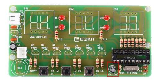
Step 15:Install 1pcs TO-92 78L05 Voltage Regulator at U2.
