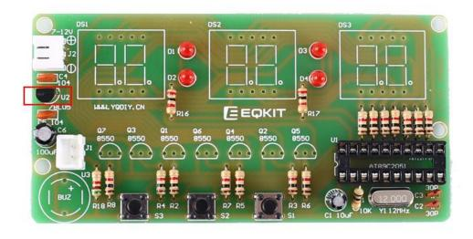
Step 16:Install 7pcs TO-92 S8550 Transistor at Q1~Q7.
