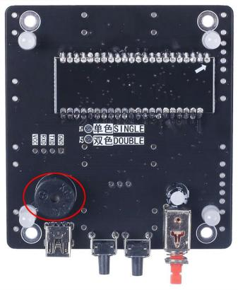
Step 8: Install 1pcs VS1838B Infrared Receiver on another side of PCB.Please do not install it on the same side as other components.
