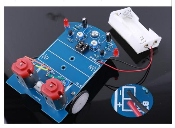
Step 28: Tear off protective film on the back of battery box and then paste the battery box on surface of PCB and pay attention to the wire.
