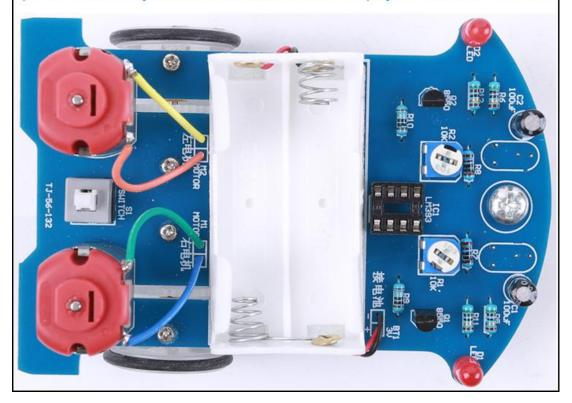
Step 29: Install 1pcs DIP-8 LM393 at IC Socket. There is a mark on one end of the IC and there is a mark on PCB where IC can place on. These two marks are corresponding to each other and are used to
