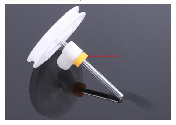
Step 18: Insert 1pcs D22mm Gear on D2\*30mm Axle and close to the D2.0mm Plastic Spacer.Note:The raised smaller gear is on the side away from the Plastic Spacer.
